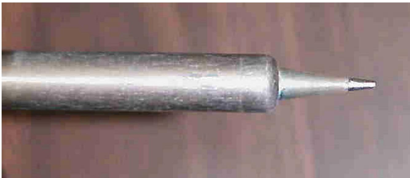
Figure 5. A properly cleaned and “wetted” soldering iron tip.
