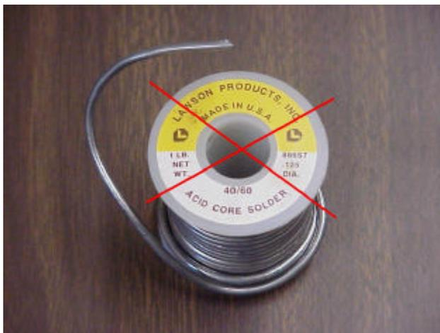
**Figure 3. Never use acid core solder for electronics assembly.**
