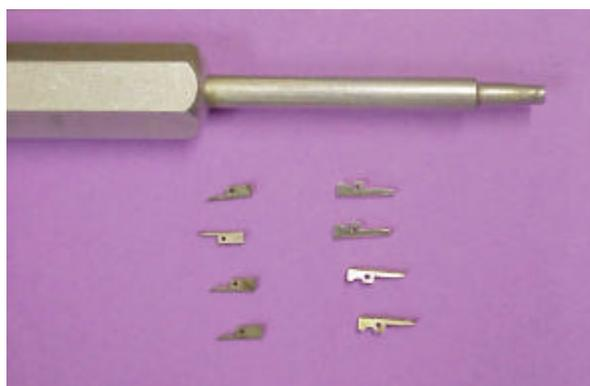
**Figure 17. Flea clip terminals and insertion tool.**
