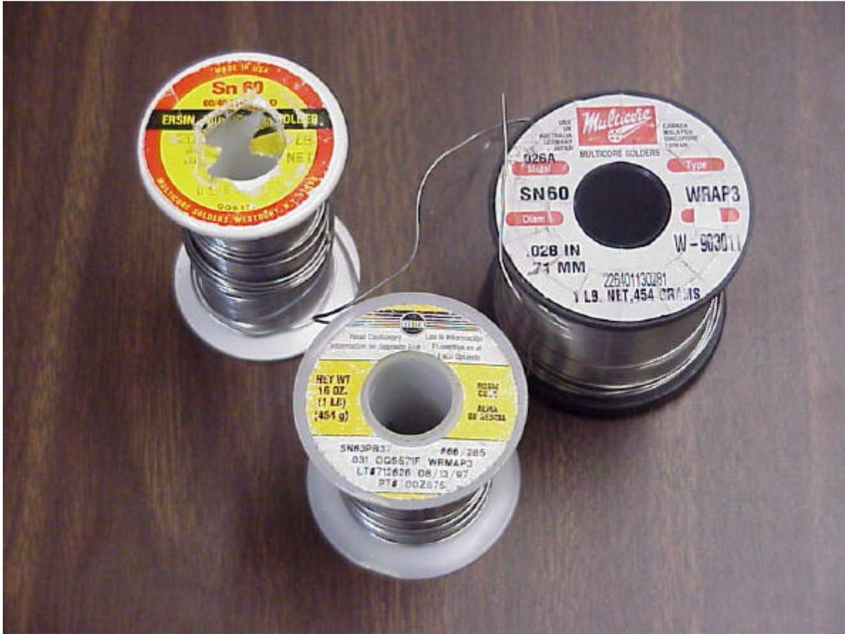
**Figure 2. Acceptable solder types (60/40 and 63/37).**
