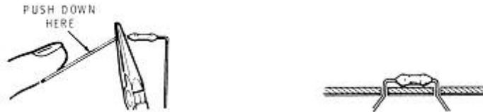
**Figure 8. Component mounting on PCBs.**
