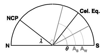
For our example of Athens, Greece, the figure above shows the range of angles to the Sun when it crosses the meridian (in grey).  $A_S$  and  $A_W$  are the altitude of the Sun at the summer and winter solstices, respectively. On the equinoxes, the Sun is on the celestial equator, so its altitude is just  $\theta$ , the altitude of the celestial equator over the southern horizon. In general:
