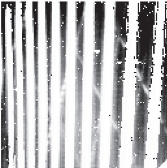
Figure 1. LH detector image ( 128 \times 128 \text{ px}^2 ) of a heavily saturated source. Vertical white bands show the 10 individual spectral orders in which the source is observed. For each spectral order, the wavelength axis is approximately vertical and the cross-dispersion axis is approximately horizontal. In the text we refer to rows and columns to describe the detector rows and columns in a given spectral order. The detector shows in this case artifacts in the form of several diagonal streaks. This artifact is different from the background gradient presented in Figure 2.
