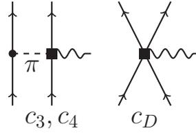
**Figure 1.** Chiral-EFT diagrams generating a two-body contribution to the weak current. The wiggly line represents the current and the dashed line the exchange of a pion.
