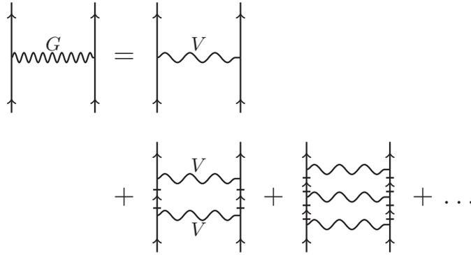
**Figure 2.** The diagrams generating the  $G$  matrix. Railed vertical lines are intermediate nucleons with very high energy. The mildly wiggly lines labelled  $V$  represent the bare interaction and the very wiggly line labelled  $G$  represents the  $G$  matrix.
