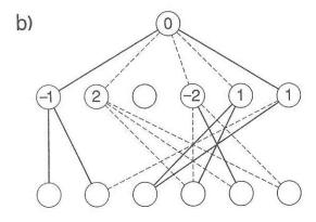
Figure 1: Typical solutions to the clump-recognition problem found by the simulated annealing algorithm. The black lines denote weights of strength +1 and the dashed lines weights of strength -1. Threshold values are displayed inside the circles corresponding to hidden and output neurons. Many of the weights are zero (absent), including one of the output weights in (b).
