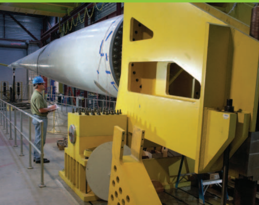
Researchers at the NWTTC conduct a fatigue test on a 37-m blade.
