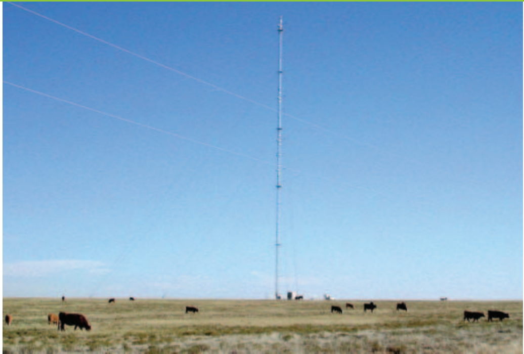
GE's 120-m (400-ft.) tower, in southeast Colorado, collected 40,000 detailed turbulence measurements to analyze.
