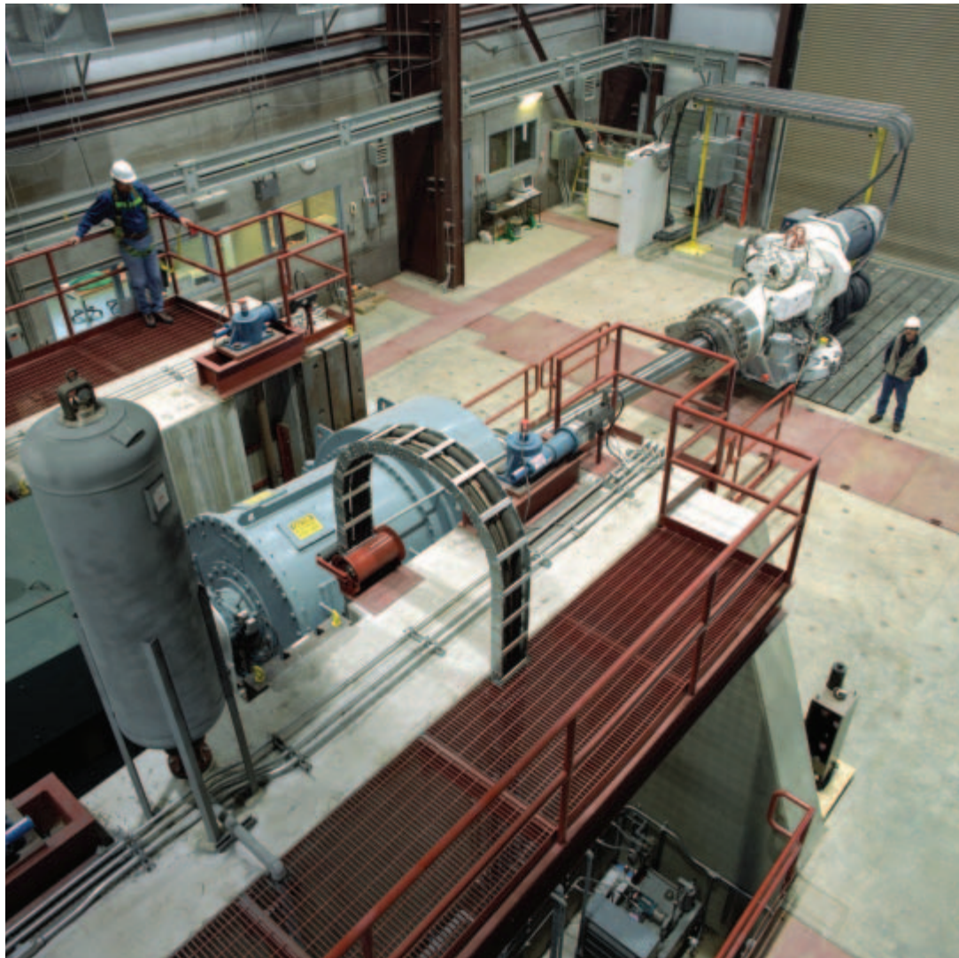
NREL's 2.5 MW dynamometer is used to conduct a range of wind industry system tests that cannot be duplicated in the field.
