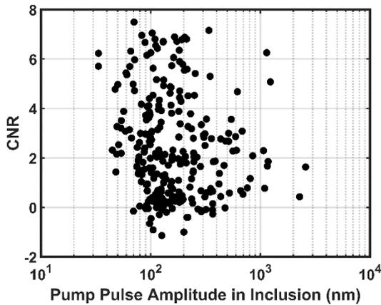
Supplemental Fig. 2. CNR of each image for which pulsatile flow was present in phantoms containing SPIO-laden inclusions plotted as a function of pump-induced vibration amplitude in the inclusion region. The correlation coefficient is -0.09 indicating no significant relationship.
