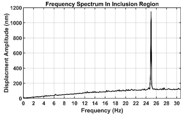
Supplemental Fig. 1. B-off displacement amplitude frequency spectrum within inclusion region of a gelatin blood vessel-mimicking phantom with a 5 kPa elastic modulus, 1 ml inclusion. A sharp peak at the 25 Hz pump pulse frequency (corresponding with a flow rate of 275 ml/min) is observed. The corresponding MMUS image is shown in Supplemental Fig. 3.
