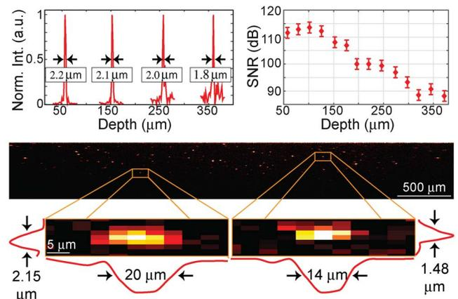
**Fig. 2.** Experimental evaluation of the parallel SD-OCT system. Top panels plot the measured axial response and SNR of a mirror at different depths. Bottom panel shows the reconstructed B-mode image of point-like scatterers. The insets show two point-like scatterers and their experimentally determined lateral and axial resolutions.
