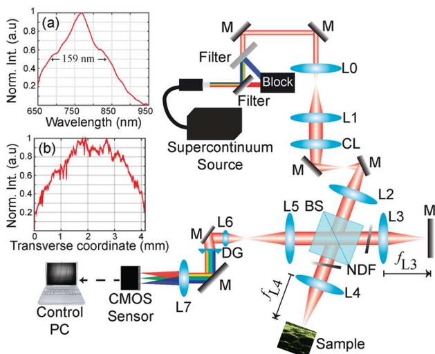
**Fig. 1.** Illustration of the parallel SD-OCT system (horizontal plane shown; see Ref. [11] for the vertical plane). M, mirror; NDF, neutral density filter; L, lens; BS, beam splitter. Panels (a) and (b) plot the spectrum and the transverse intensity distribution of the beam, respectively, both at the sensor plane with the sample arm blocked.
